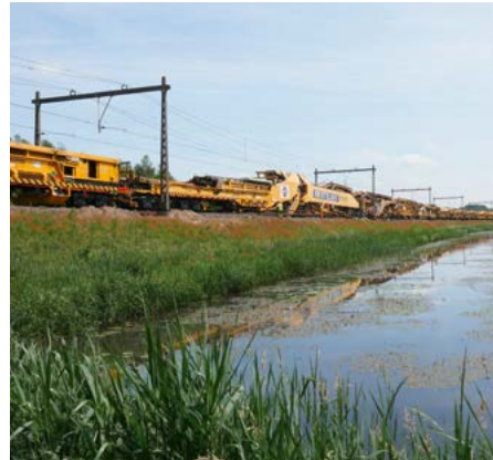
Track construction (RU 800 S), Wadden, Netherlands
